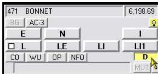
You will then get the following block where you have to enter the orientation of the part (horizontal or vertical), the size of the dents and how many dents there are on the panel. The system will then automatically calculate the required repair time for the damage.
